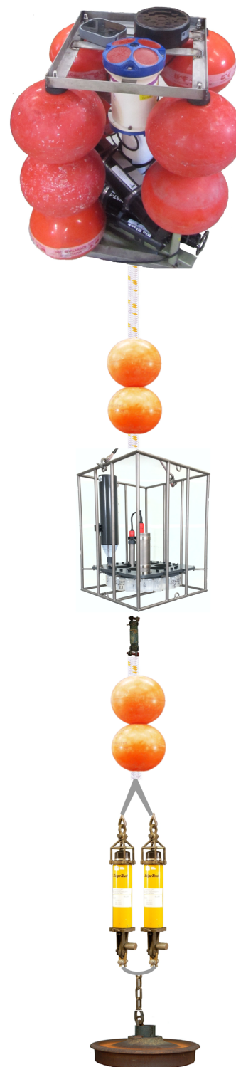
Figure 4 (right). Configuration of the second CEO mooring, showing the acoustic releases (yellow cannisters), sediment trap (frame) and the upper instrument package that houses acoustic and optical sensors. Orange and red spheres are hard plastic buoyant floats.
